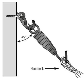
For sturdy masonry walls (not air/hollow/single brick or besser block) a 10mm dyna bolt with a large washer and rope can be used.
